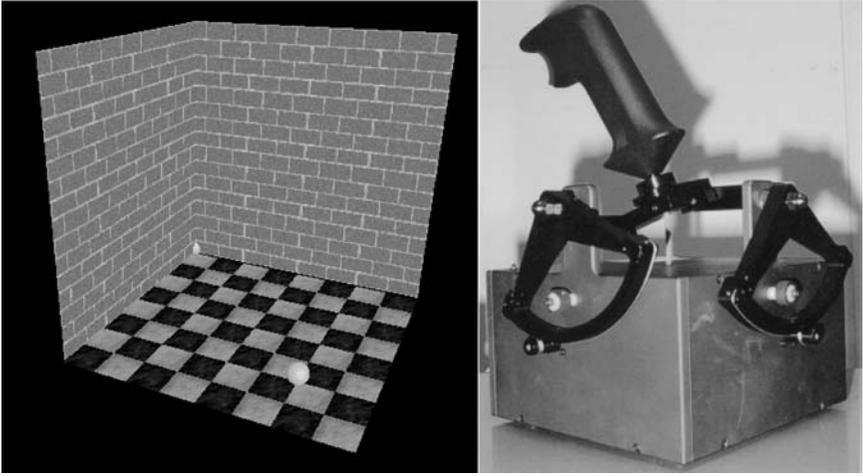
FIGURE 3 The experimental setup. A screenshot of the graphics display used in the experiment, and the force-feedback joystick (Immersion, 2001) used to control the motion of the sphere.
