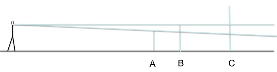
Here is a side view of a person looking at different height posts in the ground. A is shorter than the eyeheight of the person. B is the same as the eyeheight of the person. C is higher than the eyeheight of the person. The horizon has to be equal to the eyeheight of the person. Be sure to understand that. See why it has to be true.
